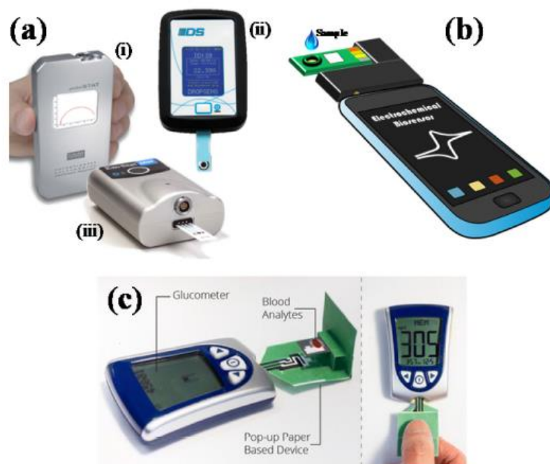
Figure 1. Portable electrochemical readers that can be employed in electrochemical biosensing. A) Commercially available pocket-sized potentiostats: i) PocketStat (from IVIUM Technologies®); ii) DropStat (from DropSens®), and iii) EmStat (from PalmSens®). B) Smartphone-based potentiostats (designed based on ref. [16]). C) Conventional glucometer adapted for other electrochemical biosensing applications (reprinted from ref. [17] with permission; copyright (2016) American Chemical Society).
