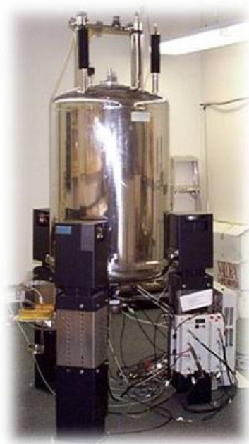
Varian INOVA-500 B_0 = 11.7 \text{ T} 499.89 MHz
